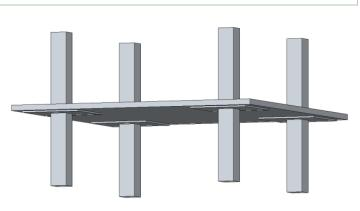
Figure 5: Flat Slab Floor System
