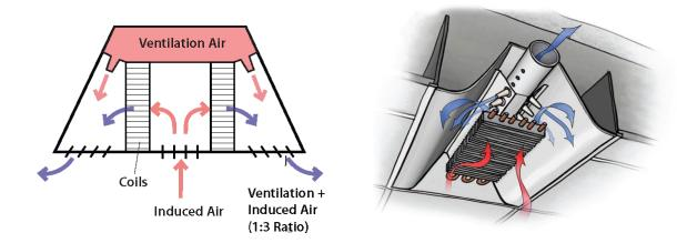
Figure 9: Active Chilled Beam Supplied with Air from AHU, image from Labs 21 Chilled Beams
