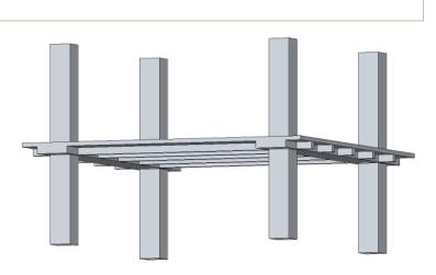
Figure 6: One-way Joist Floor System
